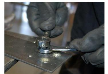
**Pictured Above:** Tool being used to install rivet nut (wrench on nut and wrench on bolt (in house we use an electric impact driver for a quick and easy install))
