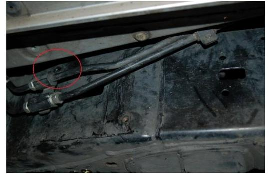
3.2 Locate and remove the bolt retaining the gas tank skid on the drivers side where the foot will need to be mounted.
