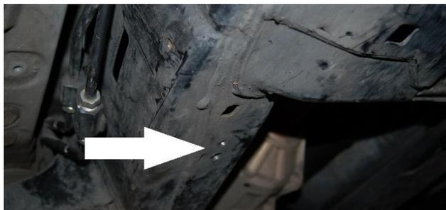
3.5 Using the provider hardware make the rivet nut installation tool to install the 3/8 rivet nuts into the 1/2 holes listed in **Step 3.5**
