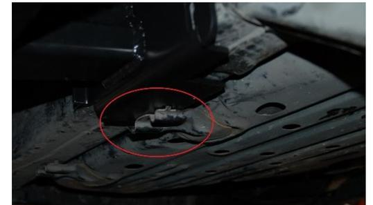
3.3 Locate and remove the bolts that retain the brake lines on the rear of both driver and passenger sides.
