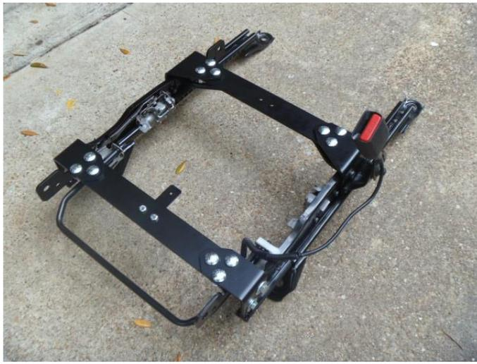
9. After the brackets are loosely bolted onto the slider track you can now move onto the vehicle occupancy sensor wiring. Please refer to the manufacturer's instructions that are provided on how to properly wire the module. \*Metal Tech 4x4 assumes no liability for the vehicle occupancy module if you choose to use one. If there are any issues or defects please refer to the manufacturer for any problems or concerns.
