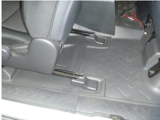
3. On the side of the seat there will be a plastic cover that will need to be removed with a Phillips screw driver. Next use your flat head screw driver to pry the plastic cover off the side of the seat
