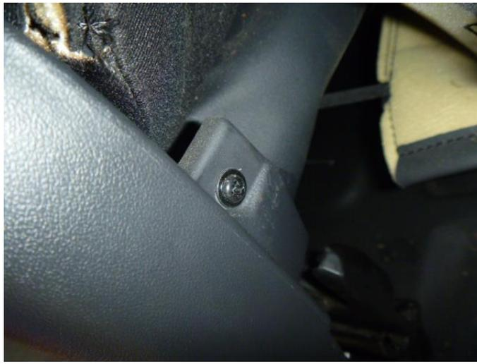
4. Next remove the 4 bolts that hold the seat in place on the floor
